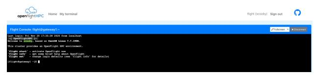
There are a few options for the terminal view, such as, making it Full Screen, changing to Zen Mode (terminal focussed with less widgets and buttons polluting the screen) and disconnecting the terminal session.
